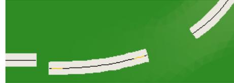
As you move the tip, the whole track flexes from end to end. The curvature of the other end is maintained until you adjust it by its tip.
