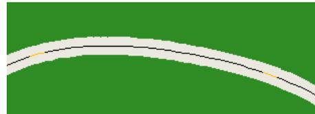
Use the “Connect Quintic Easement, between ends” tool to produce a very smooth curve that gradually eases one radius into the other. The transition curve that resulted is not a unique solution to the overall problem, though. Let’s try the same situation, with a slightly different end for the left curve.
