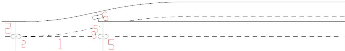
The build process recognized the two splines attached to the turnout overlapped. It trimmed the splines so that the spline proceeding from the non-routing side of the turnout was left intact at its assigned width of 3”. During the build, the turnout spline (Spline 1) and Spline 5 were subtracted from Spline 6. While this could be built with connectors by gluing the three pieces together, it is possible to make a composite Roadbed Spline that simplifies building.
