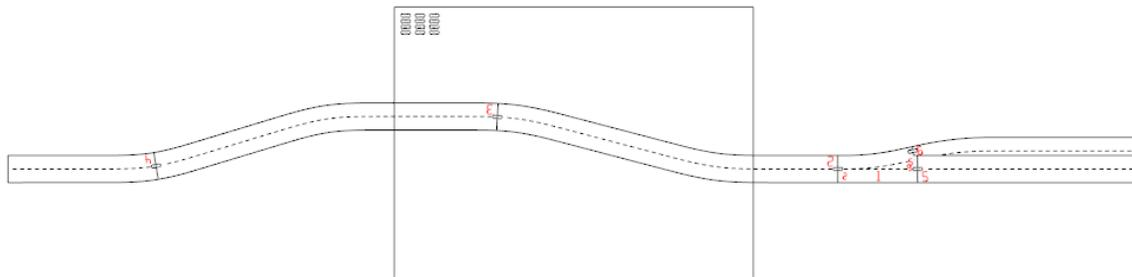
The difference in width is obvious when compared with the Track Splines built previously. The splines in the open area on the left are fine, but the area around the turnout needs attention. What should be done?
