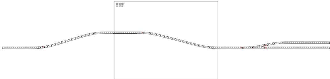
The large box is the size of the material that can be handled by the cutting tool. A set of connectors is in the upper-left of the material box, grouped so they can easily be relocated as a set. We also see the Track Splines that have been built. Note that only the Layout Splines layer is active and displayed. It's easy to toggle **Layout Splines Only** mode: View / Show / **Layout Splines Only** (Ctrl+F12). With the select tool, move the splines into the material box in a compact arrangement.
