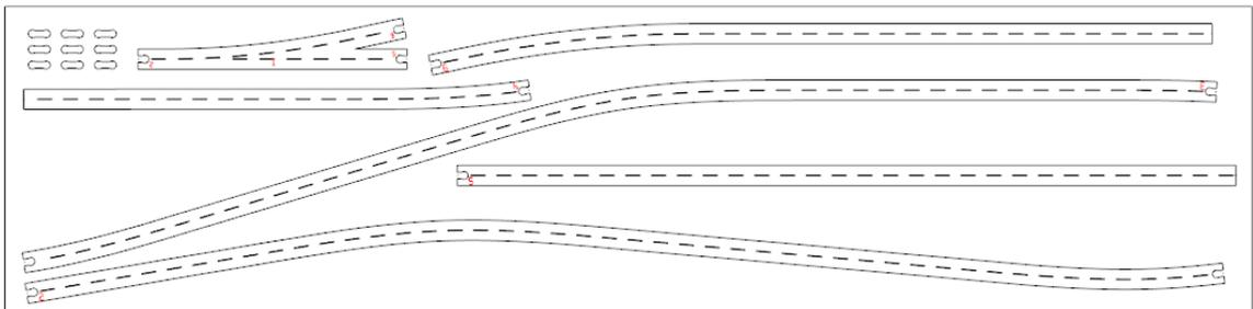
This is a nice, efficient arrangement of the pieces. The bottommost spline was rotated about 160 degrees from its original position to make good use of material. The less material you use, the less you'll pay for your Layout Splines. Make sure to leave at least 1/8" between adjacent splines for the cutting tool.
