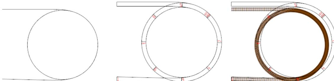
The original track centerlines are shown on the left. The center image shows 3" Roadbed Splines built from the track and the right images shows the track with rails and ties superimposed on the Roadbed Splines. Note now the splines do not overlay the track as one might expect. That's because the very steep grade had to be accounted for when building the splines. Without compensating for grade, the splines would be too short and serve no purpose.
