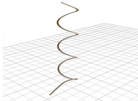
This example uses a helix with a grade that could not possibly work on a model railroad, as shown at the right. The purpose of the example is to show the grade compensation performed when building Layout Splines and the appearance of splines built on grades when viewed in 3D. With typical grades, the differences will be far less pronounced.
