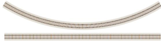
But what happens if we build Roadbed Splines? Here, the width setting **Roadbed** was chosen, using the Main Layer roadbed width of 3" as the spline width. The output of the build is shown in the left image.
